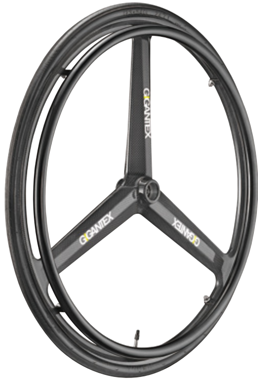
24" Carbon three spoke wheels Weight : 2000g
